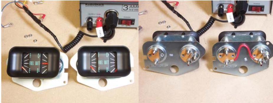
How to tell the difference with visual inspection? The Ammeter is on the Left, and the Voltmeter on the Right. Notice that the ammeter pointer centers at rest, and the voltmeter pointer drops below the bottom picket. On the back side the ammeter has two Hot wires that are both insulated from the case, while the voltmeter is pre-wired off the fuel gauge and grounded to the case.
