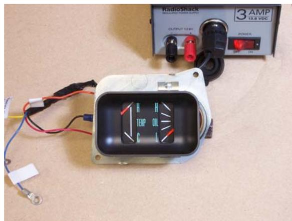
5. Temperature Gauge No Signal from Sender.
