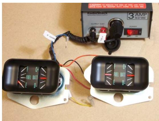
On the left is an ammeter gauge shown at rest....or when the battery is charged [Normal Driving].
