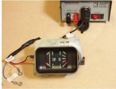
6. Temperature Gauge No Ground. Pointer moves up and out of sight.
