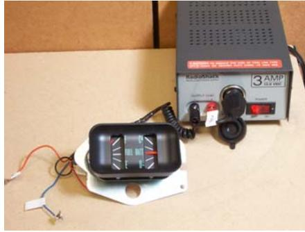
6. Fuel Gauge ...No Signal from sending unit ... The Pointer travels up past Full and out of sight.
