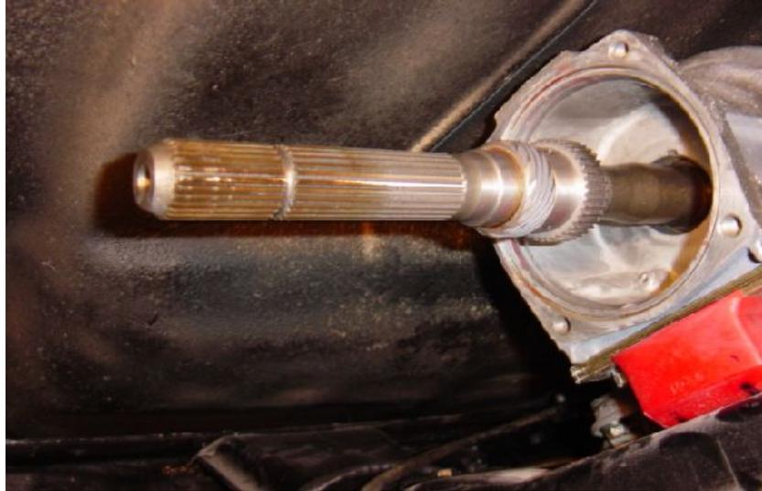
Slide tail housing into transmission until seated and visually confirm that the drive gear of the assembly is centered in sleeve opening. See picture below.
